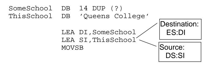
To move an entire string, the CX register is loaded with the length of the string and the REP prefix is used.
